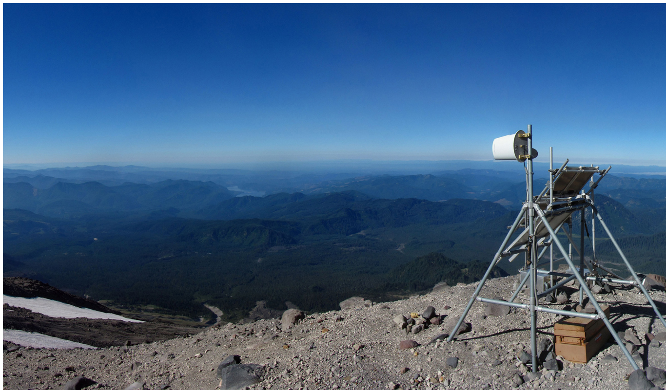
Scientists rely on remote monitoring equipment, like this station on the southwest flank of Mount St. Helens, to monitor volcanic activity. These monitors deliver real-time data around the clock. Volcano monitoring stations integrate many instruments into a single package to lower power requirements, reduce instrument footprint on sensitive landscapes, enable rapid deployment, and transmit data effectively under extreme weather conditions. Image: U.S. Geological Survey.
