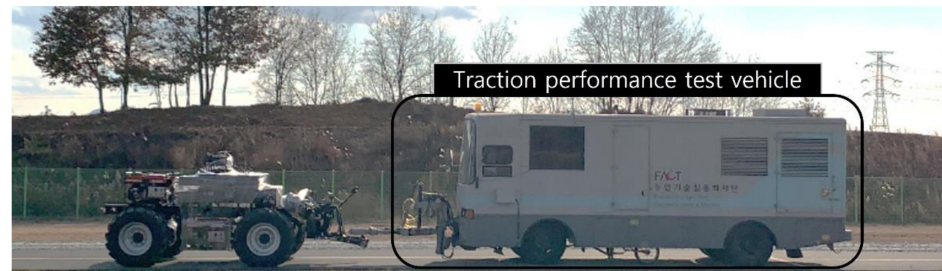
Figure 4. Traction test of the electric AWD tractor using traction performance test vehicle on a concrete surface.
