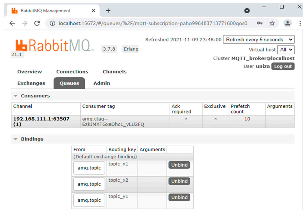
Figure 10. RabbitMQ queue setting for virtual redundant sensor as a consumer.
