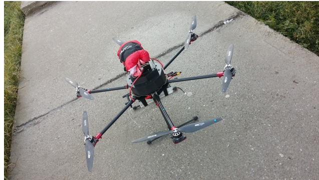
Figure 4. Hexa-rotor aerial copter design.
