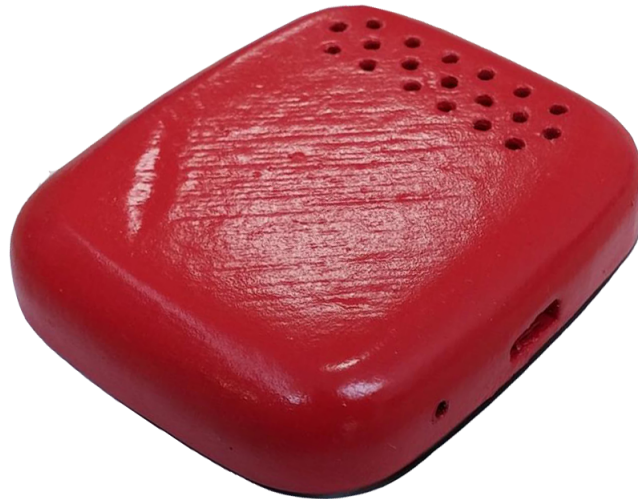
Figure 2. Special mounting unit designed for the sensing unit.
