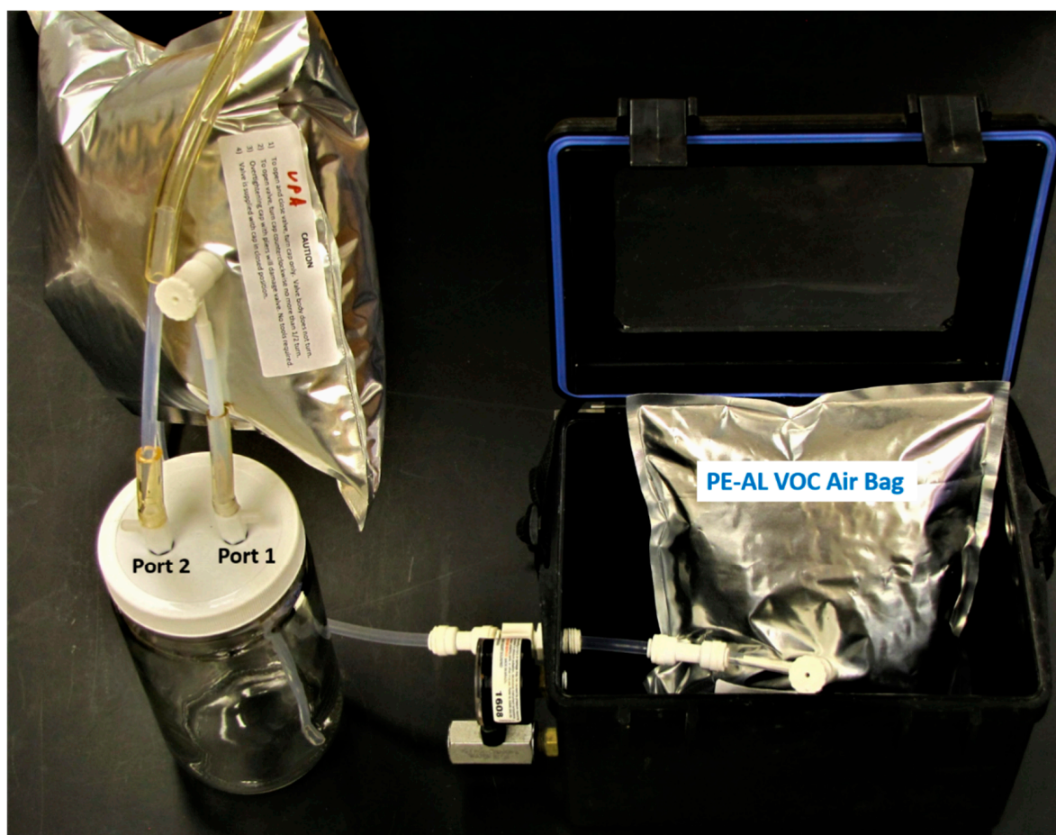
Figure 1. Bat VOC air-collection apparatus assembly. Xitech vacuum chamber (at right, containing PE-AL VOC air-sampling bag inside) with glass bat air-sampling chamber (at left) connected via two port valves to FEP tubing with Port 1 (receiving air inflow from pure zero-air replacement bag), and Port 2 (allowing outflow of bat sample air to input port of Xitech air-collection chamber and internal VOC air-collection bag).
