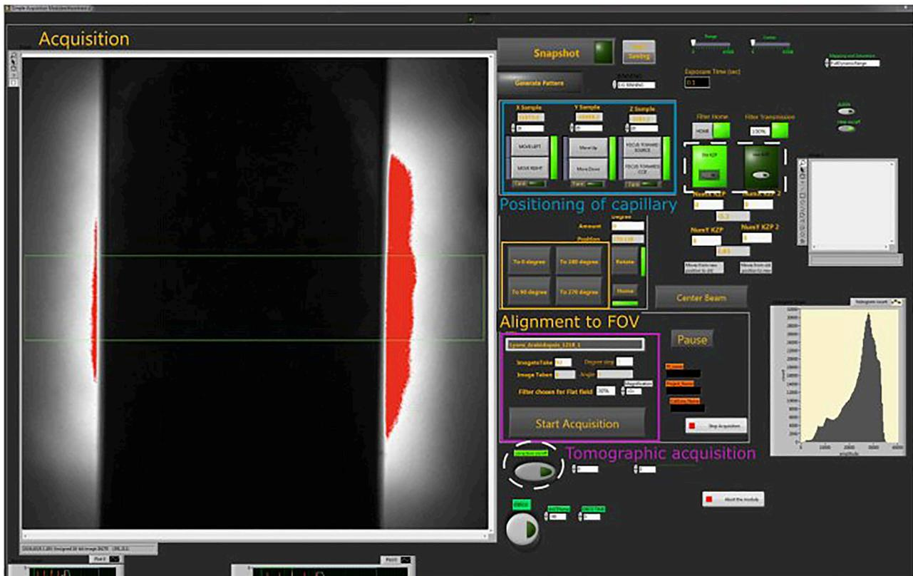
**Figure 6. Graphical User Interface for the tomographic data acquisition**
