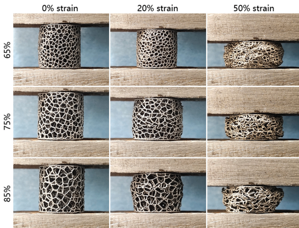
Figure 8. Geometric morphologies of trabecular Ta scaffolds with porosities of 65%, 75%, and 85% under strains of 0, 20%, and 50%, respectively.
