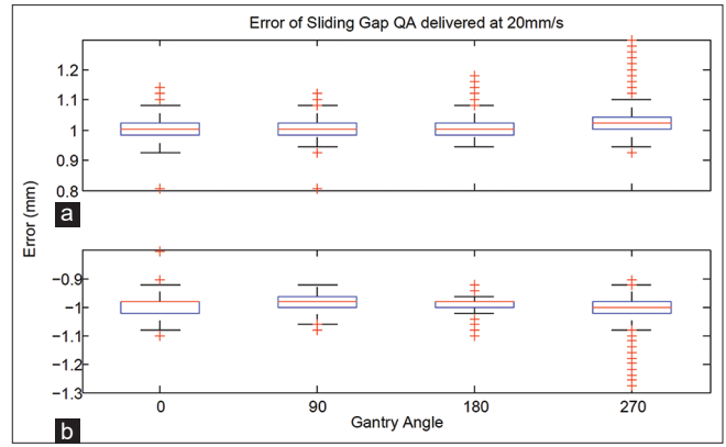
Figure 3: Box and Whisker plots of the multileaf collimator error of Sliding Gap QA (20 mm/s) performed at cardinal gantry angles. The error (mm) for Sliding Gap QA delivered at four different gantry angles on iX-2 for (a) bank A, and (b) bank B. Leaves moved with velocity 20 mm/s. The box and whisker plot represents the data as follows: The top line (or whisker) is the maximum value, the next line is the 3 rd quartile, the red line is the median, the next line is the 1 st quartile, and the last line is the minimum value. The red crosses are outliers
