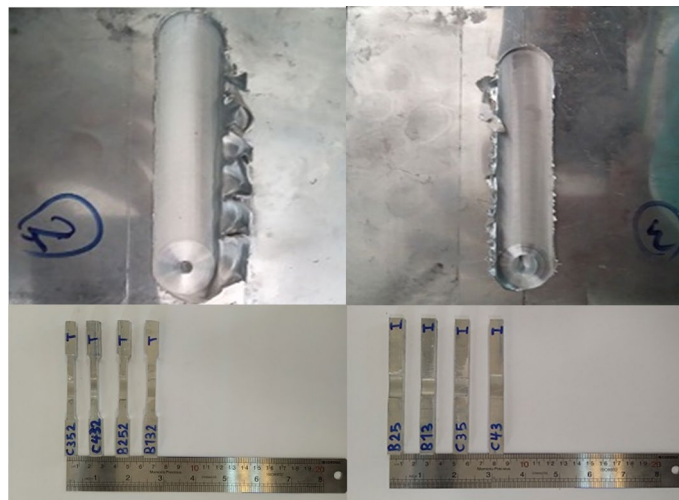
Figure 13. The welded specimens with the optimized welding values.
