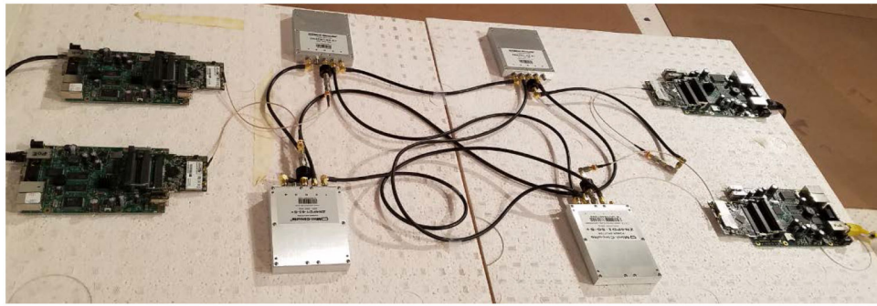
Figure 1: Wireless coexistence testing using a conducted test method. (a) Setup diagram. (b) Lab deployment.
