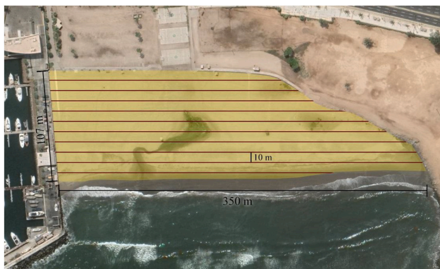
Fig. 1. Map of a sand beach displaying the sampling area (yellow area) and appropriate transects parallel to each other (red lines) separated by 10 m, as described by De-la-Torre et al. (2021b). (For interpretation of the references to color in this figure legend, the reader is referred to the web version of this article.)
