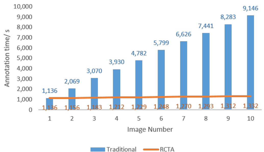
Figure 4. Annotation time performance comparison between RCTA and traditional annotation method. The blue bar represents the time used for the traditional annotation method, and the orange line represents the time used for the RCTA annotation method. The traditional method needs to manually annotate all targets, but RCTA only needs to remove the redundant annotation boxes for augmented images, so the annotation time of RCTA is reduced by over 80% compared to the traditional method as the number of images increases.
