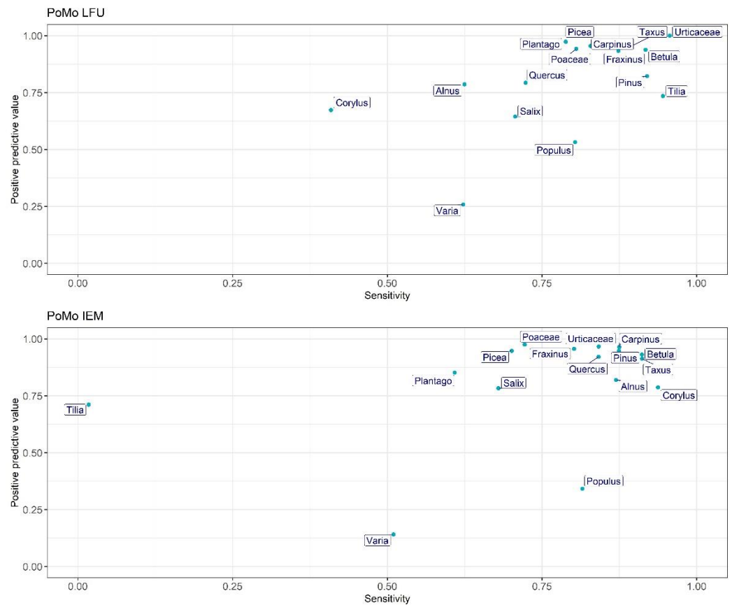
Figure 5. PoMo capability of identifying different pollen types. Sensitivity in the X-axis shows the percentage of correctly identified particles. The positive predictive value (PPV) in the Y-axis shows the ratio of automatic identifications that were correct.
