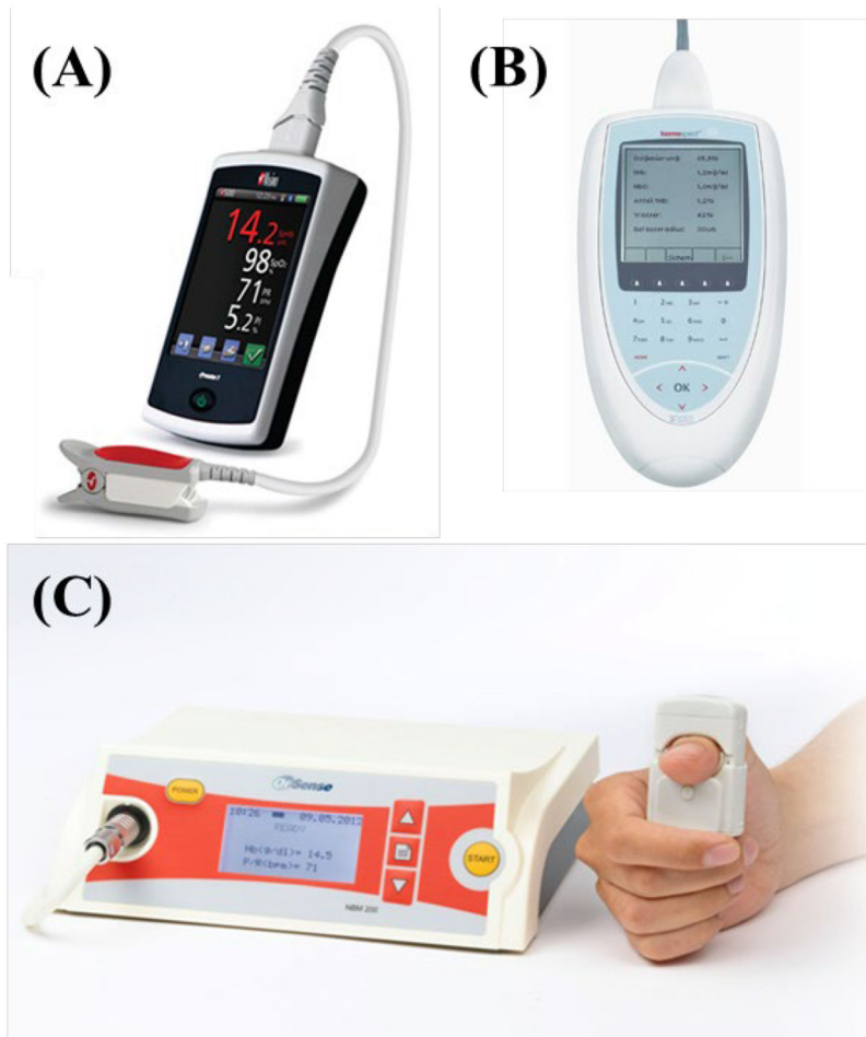
Figure 2. Non-invasive point-of-care Hb level measurement technologies. (A) Pronto-7 ® (Reproduced from online resource [231], Masimo, Inc), (B) Haemospect ® (Reproduced from online resource [232]), and (C) NBM-200 (Reproduced with permission from OrSense U.S., LLC)
