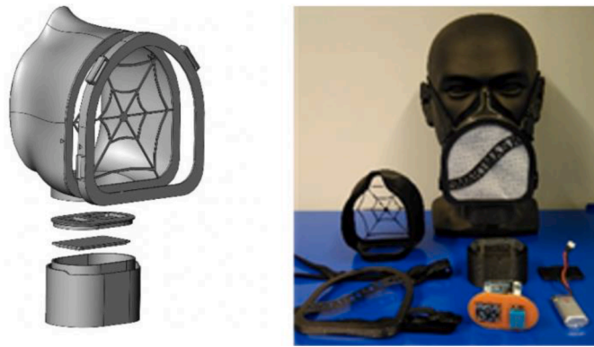
Fig. 1. a) Design image of the assembly of the 3D-printed mask. b) 3D-printed early prototype of the Smart Mask on the model head and disassembled version of the mask in front.
