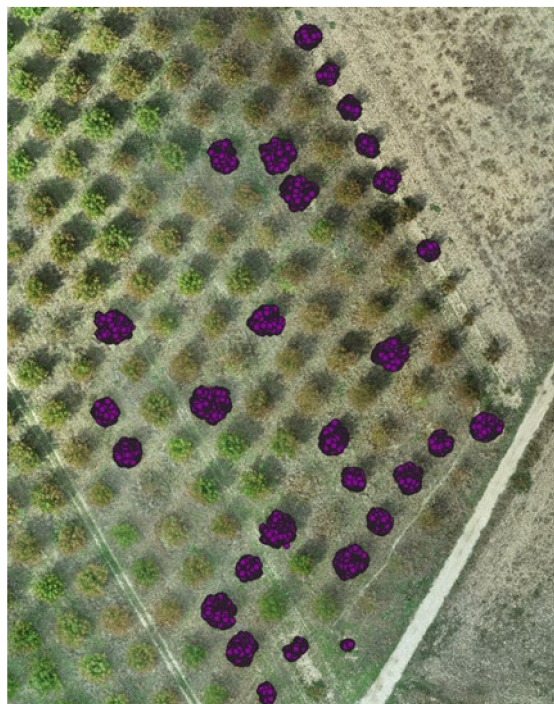
Figure 4. The projection of the point cloud (top view) of the orchard in 2D, mapped with the two methods used in the study; the ground-based system using depth camera mounted on Thorvald UGV and the orthomosaic exported from aerial images acquired using UAV.
