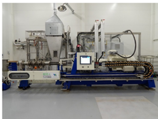
Figure 1. Extruder Clextral Evolum EV 53 for polyphenol extrusion-extraction.
