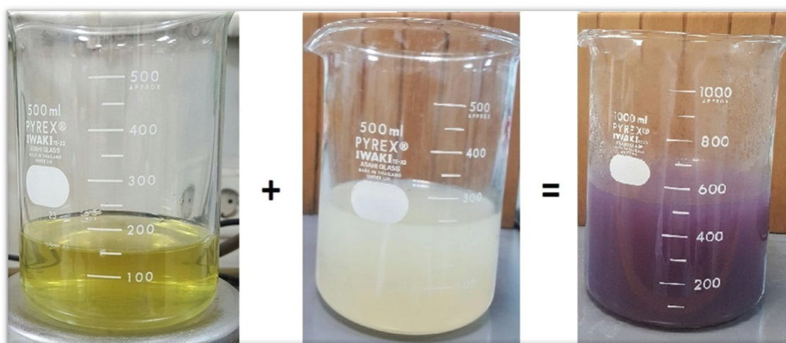
Figure 3. Yellow colored solution is Chloroauric acid, white colored solution is seed extract of Citrullus colocynthis , which when reacted then turned purple-colored, indicating the formation of AuNPs due to capping or reducing agents.
