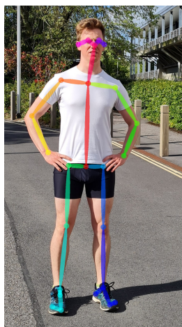
Figure 3 Twenty-five keypoints detected using the OpenPose pose estimation algorithm (Cao et al., 2018) applied to a single image.
