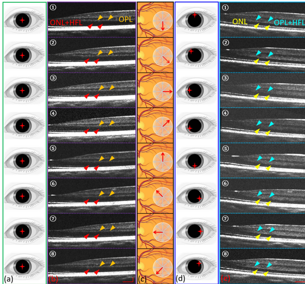
Fig. 5. (a) Incident beam entry positions in the regular spoke scanning pattern. (b) Eight selected cross-sectional scans (every 45^\circ interval in a scanning cycle) acquired by the regular spoke scanning pattern. Red arrows indicate the combined layers of ONL and HFL. Orange arrows indicate the OPL. (c) Illustration of retinal spoke scan. (d) Corresponding incident beam entry positions in the spoke-circular scanning pattern. (e) Eight selected cross-sectional scans (every 45^\circ interval in a scanning cycle) acquired by the spoke-circular scanning pattern. Yellow arrows indicate the ONL. Cyan arrows indicate the combined layers of OPL and HFL. Scale bars in (b) and (e) are 300\ \mu\text{m} (horizontally) and 100\ \mu\text{m} (vertically).
