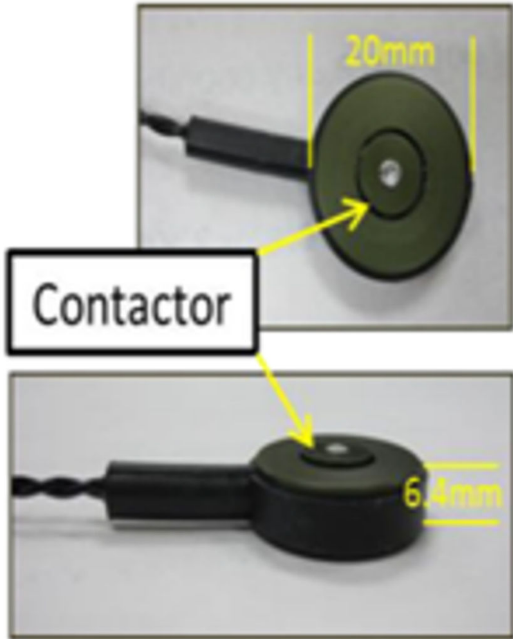
Fig. 3. The vibrotactile device (C-3 Tactor). The contactor is the vibrating part in contact with the skin.
