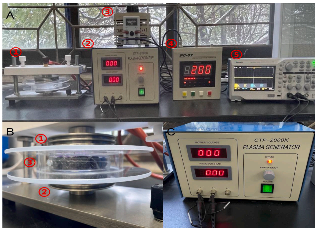
Fig. 1. Schematic diagram of the CP equipment. (A) The schematic diagram of each component in the system. 1 is the DBD reactor; 2 is the plasma generator; 3 is voltage booster; 4 is digital pulse wave generator; 5 is the digital oscilloscope. (B) DBD reaction system. 1 is a high voltage electrode; 2 is a low voltage electrode; 3 is a quartz reaction chamber. (C) The plasma generator.
