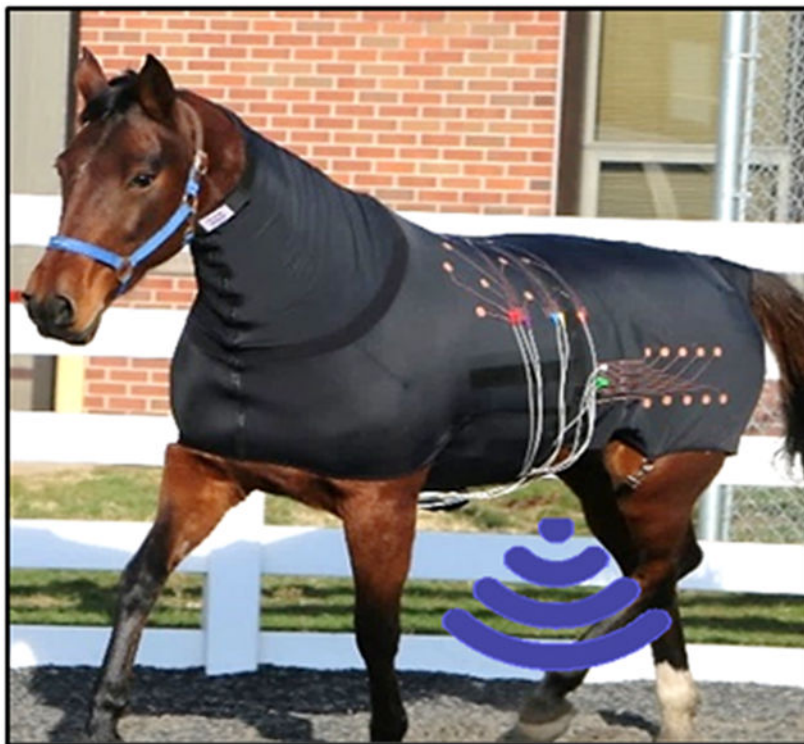
Horse in a custom e-textile under ambulatory conditions for remote health monitoring.
