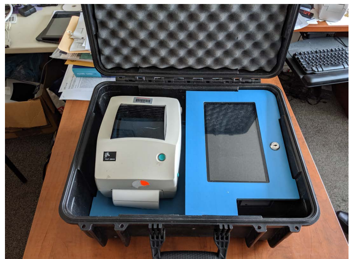
FIGURE 1 Portable field unit with thermal printer and touchscreen installed in case.
