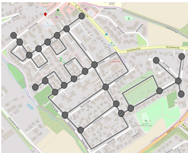
Fig. 3 Map with vertex-edge graph of the road network (Map by Openstreetmap, licence CC-BY-SA 2.0)
