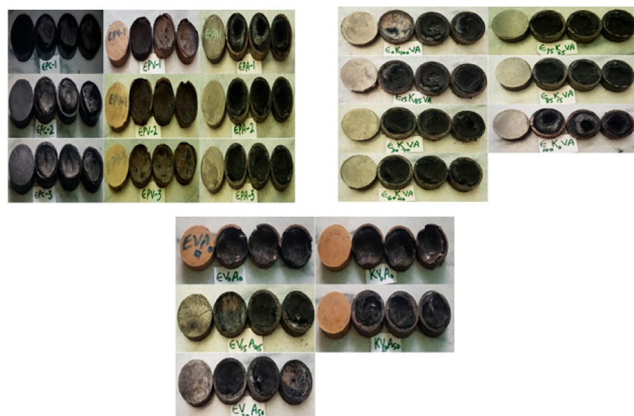
Figure 2. Top: Dumbbell-shaped samples before and after mechanical testing. Bottom: The samples before and after ablation rate test, where each sub figure represented first sample before and remaining three samples after ablation testing.
