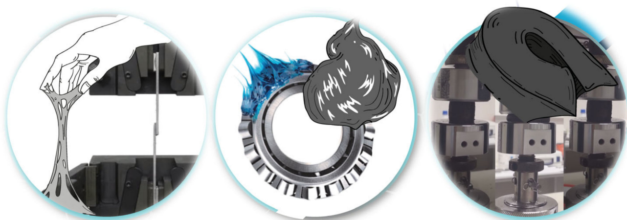
Figure 4. Main bio-polyurethanes studied, i.e., adhesives, lubricating greases and elastomers, from left to right, with testing or application as background.
