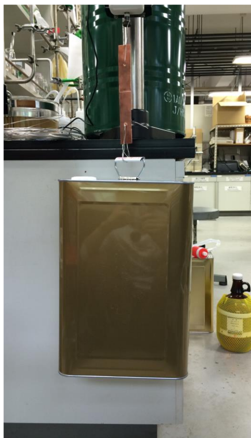
Figure 10. Photo image of aluminum plates adhered with NPDG and DETA (curing time = 6 h, 25 °C, [amine]/[epoxy] = 1/1) loading a can containing 11 kg of hexane.
