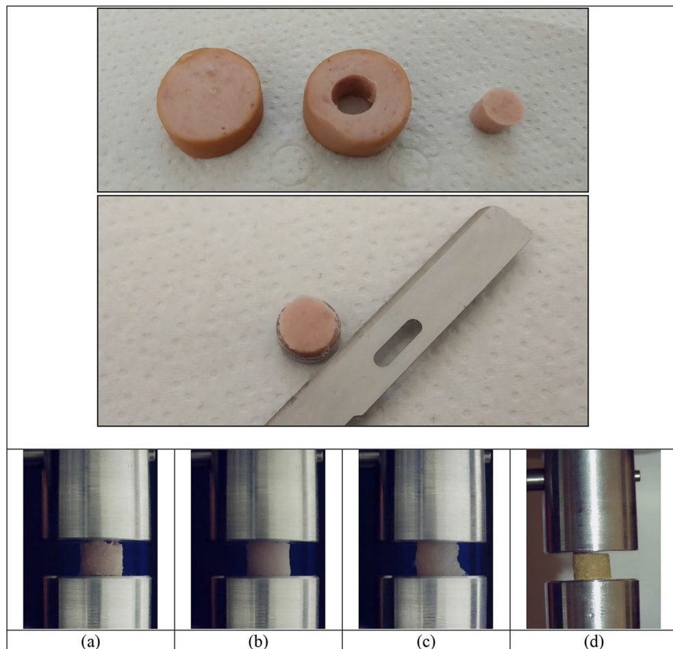
Figure 1. (Top) Process for obtaining the samples. Obtaining a cylinder using an 8 mm punch and placing it on the apparatus to fix its thickness by cutting it to the desired thickness. Process example shown correspond to a sausage. (Bottom) Images correspond to tested samples of Frankfurt style sausage (a), processed turkey (b), non-processed chicken (c) and cultured meat Frankfurt style sausage (d).
