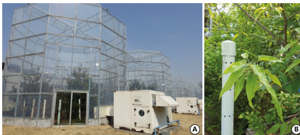
Fig. 1. (A) Open top chambers at the National Institute of Forest Science in Suwon, Korea and (B) its internal view showing a CO 2 injection nozzle and plants. Permitted from Kim et al. 34
