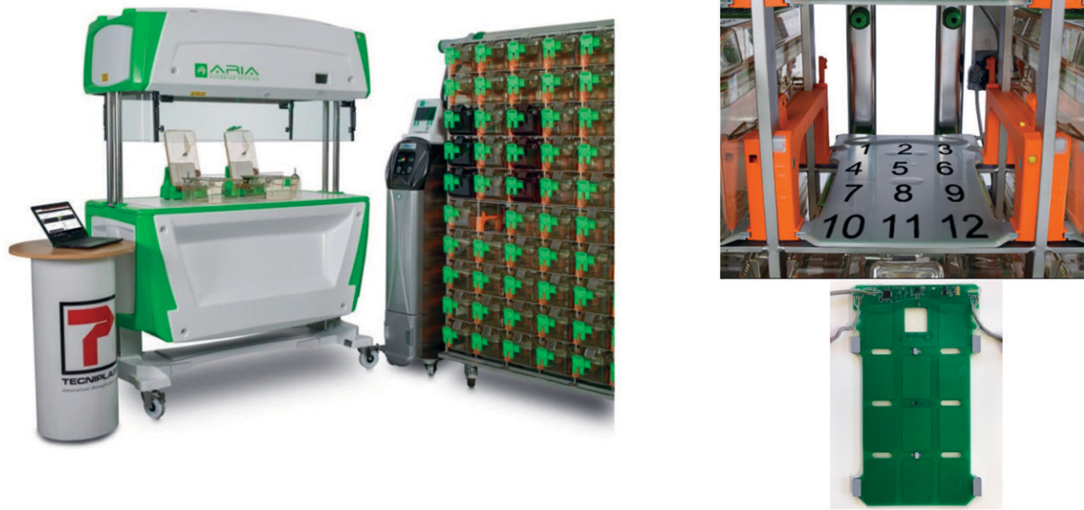
Figure 1. The digital ventilated cage system is an automated home-cage monitoring that continuously records spontaneous activity in the cages. The system can collect data from thousands of home cages simultaneously.
