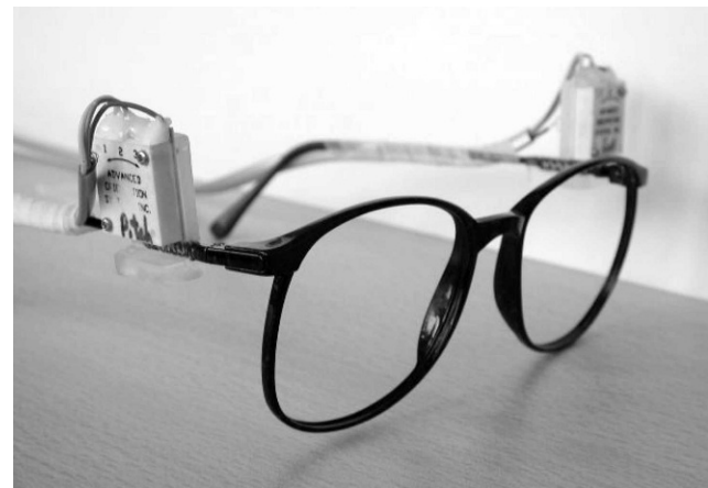
Figure 2. Cranial portion of device. Note placement of inclinometers on opposite sides.
