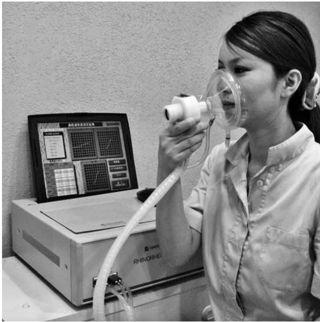
Figure 1. Anterior rhinomanometry device for measurement of nasal airway resistance (RHINOEOGRAPH MPR-3100, Nihon-Kohden Co, Ltd, Tokyo, Japan).
