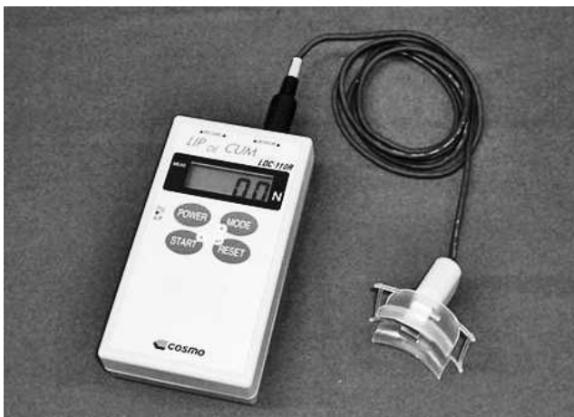
Figure 2. Full view of strain measuring device for maximum lip-closing force (LIP DE CUM LDC®-110R, Cosmo-Instruments, Co, Ltd, Tokyo, Japan).
