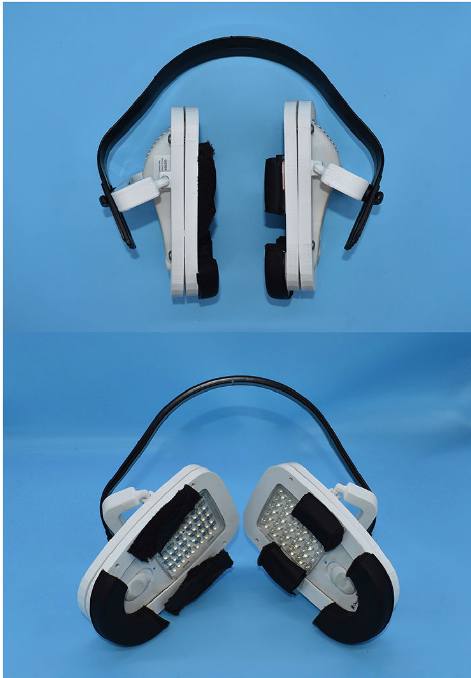
Figure 2. Custom-designed headset containing an LED-RL treatment device and mock phototherapy device on opposing sides.
