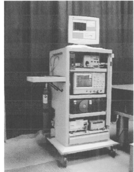
FIG. 1. (a) Schematic diagram illustrating the modular tr-LIFS apparatus setup; and (b) photograph of the system hosted in a mobile endoscopic cart; PMT: multichannel plate photomultiplier tube; ICCD: intensified charge-coupled-device camera.
