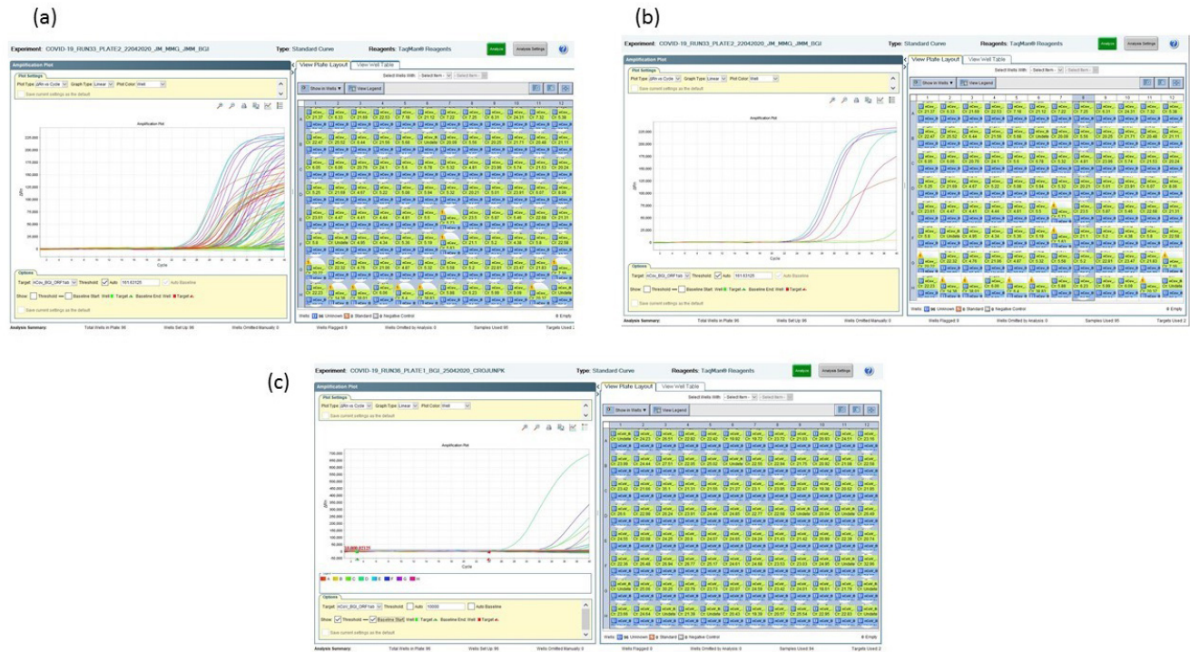
Figure 2. BGI assay performance. (A) Multicoloured amplification curves at 0.5X of the manufacturer's recommended volume indicating a majority positive results from a 96-sample test run. (B) Selection of a single column highlighting 6 out of 8 samples were positive for SARS-CoV-2. (C) Re-run of the same samples from B with 0.375X of the manufacturer's recommended volume and 0.25 \mu l of the enzyme mix only detected 4 SARS-CoV-2 positive samples at a Ct value cut-off of 34.
