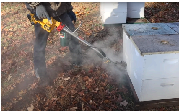
Fig. 1. An adapted amalgamation of a leaf blower, propane gas heater, and oxalic acid vaporizer as developed by a commercial beekeeping operation to improve the economic viability of acute oxalic acid treatment of many hundreds of colonies. Devices such as this allow even large apiaries to be treated with minimal labour (relative to the wider context of beekeeping), but rely on beekeeper-led innovation and potentially loose regulatory environments.
