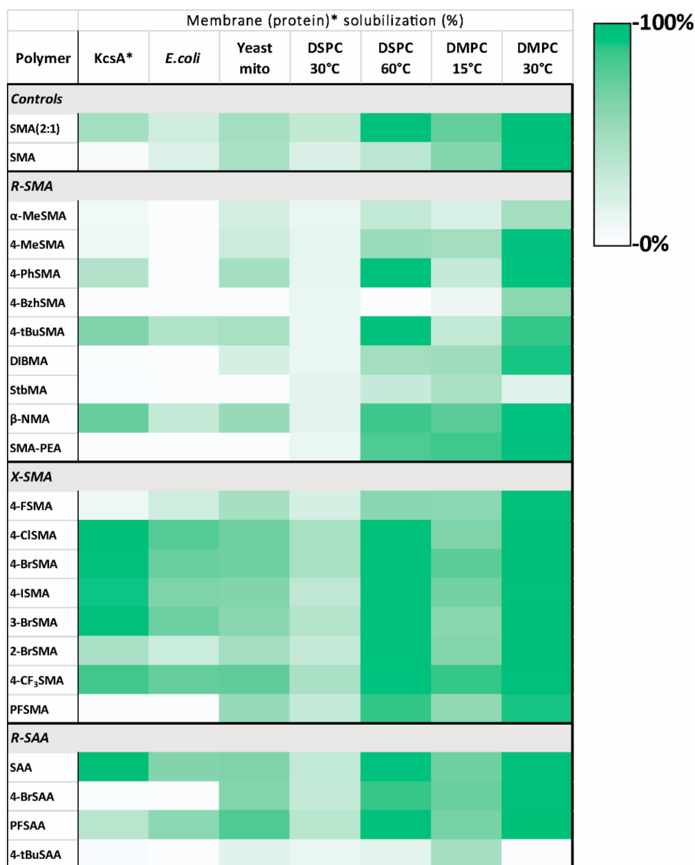
Figure 6. Heatmap summarizing membrane solubilization properties of the polymers in the copolymer library in different membrane systems. KcsA membrane protein solubilization is based on densitometric analysis of protein bands on SDS-PAGE, i.e., the percentage of KcsA extracted. Solubilization of all other (whole) membranes is based on turbidimetric analysis with the percentage of solubilization given as a relative decrease in OD.
