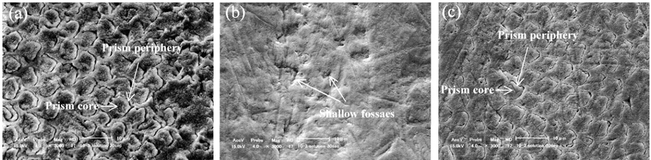
Figure 2. SEM photomicrographs of etching efficacy. (a) Superbond etching. (b) Superbond self-etching primer. (c) Transbond Plus self-etching primer.
