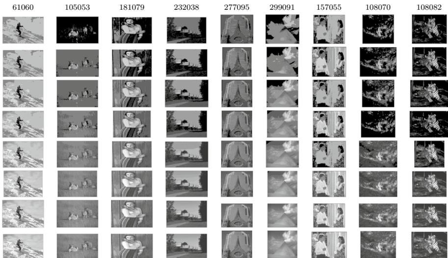
Fig. 20 The segmented images were obtained by the proposed algorithm using threshold levels 2, 3,4,5,10, 20, 40, and 100, respectively
