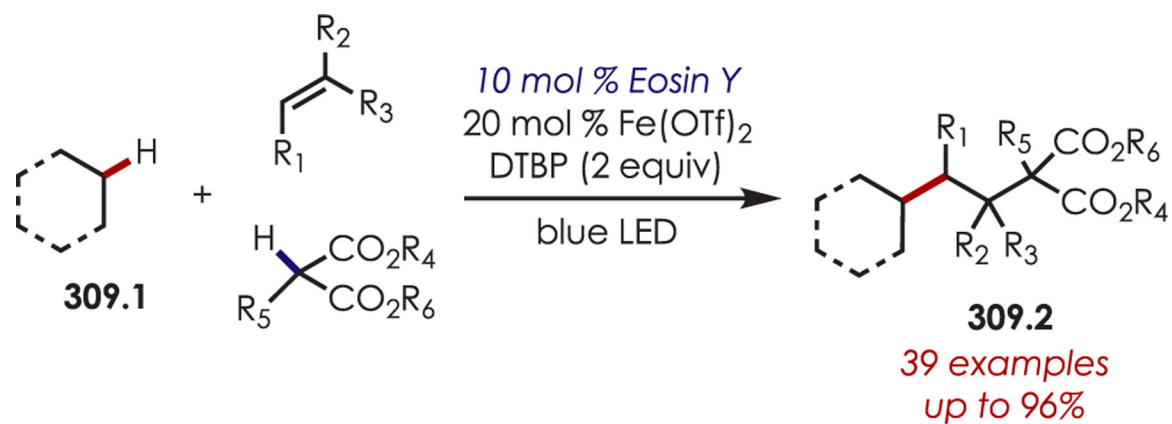
Scheme 309. Dialkylation of Alkenes with Two Distinct C–H bonds by Dual Photoredox and Iron Catalysis
