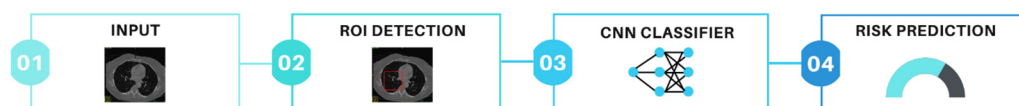
Figure 5. Example of an ‘end to end’ cancer detection pipeline. 1: A whole CT volume is used as input into the model. 2: A region detection architecture (such as UNet) is used to identify a sub-volume and assign a bounding-box ROI. 3: The volume encompassed by the ROI is input into a classification CNN (such as InceptionNet) to learn patterns associated with the outcome variable. 4: A risk prediction of malignancy is output. Abbreviations: ROI: region of interest, CNN: convolutional neural network. CT images taken from the public LUNGx dataset [97].
