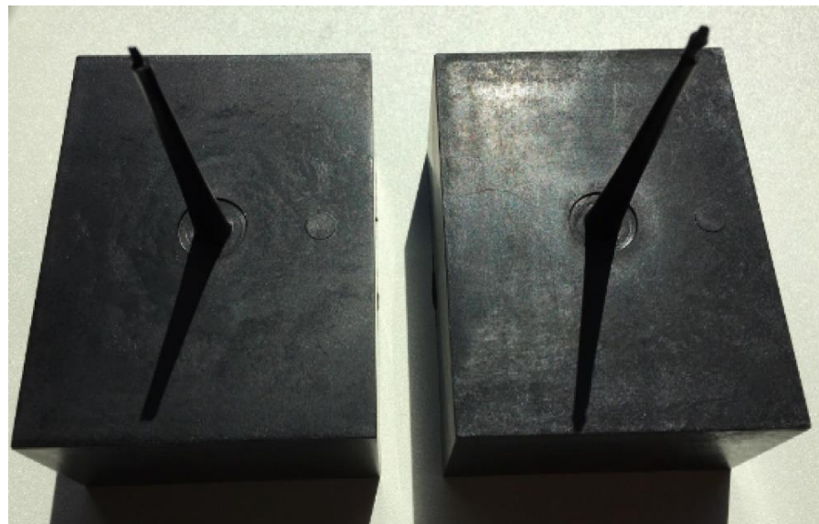
Figure 9. (Left) solid and (right) MIM box-shaped parts.
