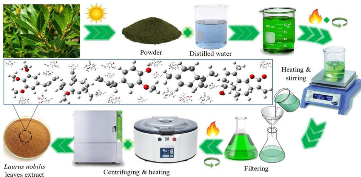
**Figure 10.** Schematic route for preparing *Laurus nobilis* leaf extract powder that was used for mild steel corrosion prevention. (Reprinted with permission from Ref. [213]. Copyright 2020 Elsevier Publications).
