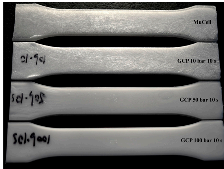
Figure 8. Surface visual quality of the microcellular molded parts at different GCPs.
