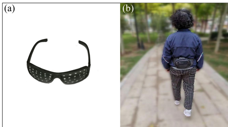
Fig. 1 a Pigmented sunglasses to simulate visually impaired walking. b A participant wore a smartphone in the L3 region of the lower back
