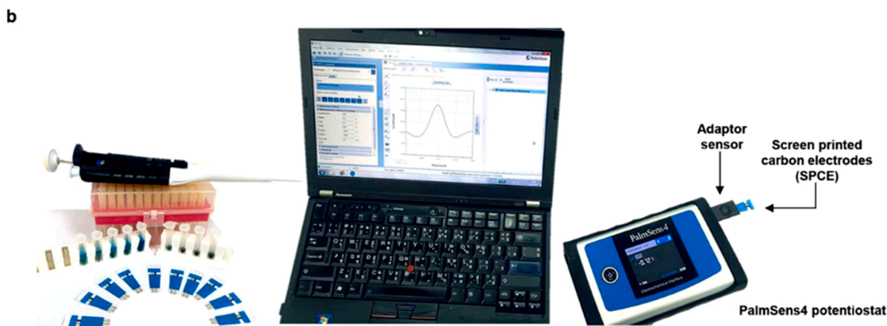
Fig. 1. a, a scheme for the extraction and analysis of SARS-CoV-2 RNA from clinical samples using the electrochemical biosensors with RCA of the N and S genes. b, The electrochemical analysis by using a portable potentiostat device connected to a laptop. Note: The N gene is the nucleocapsid protein for RNA packaging and viral particle release.
