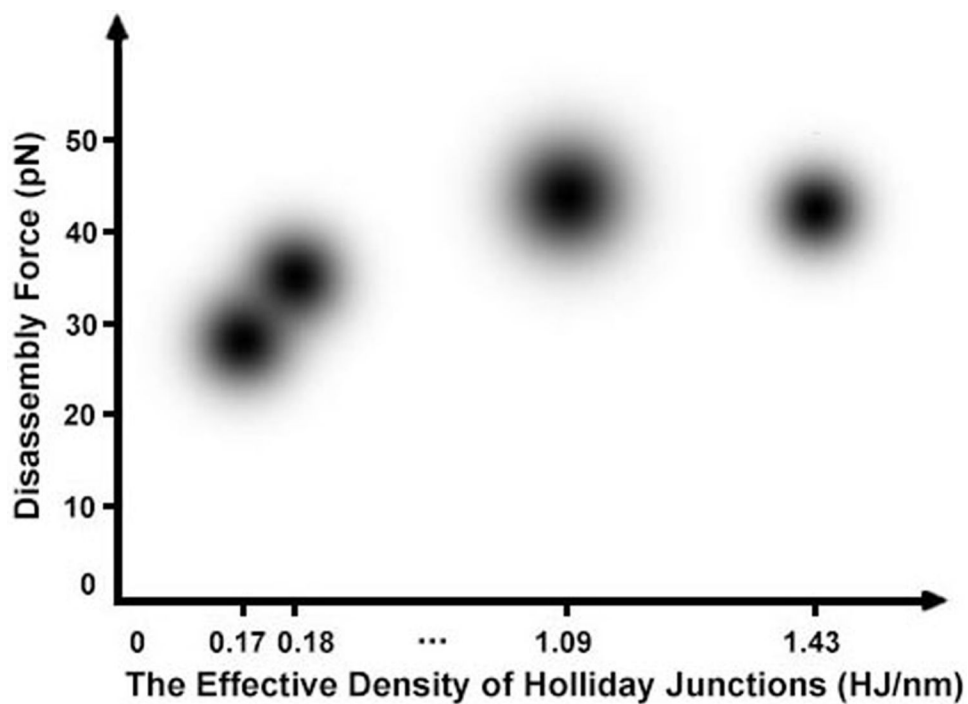
Fig. 15. Relationship between disassembly force (pN) of DNA origami nanoassemblies and densities of Holliday Junctions ( \text{HJ nm}^{-1} ) along the direction of applied force. This plot uses published data. 24
