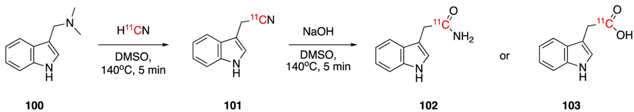
Fig. 16. Synthesis of 3-indolyl[1- 11 C]acetic acid ( 103 ).
