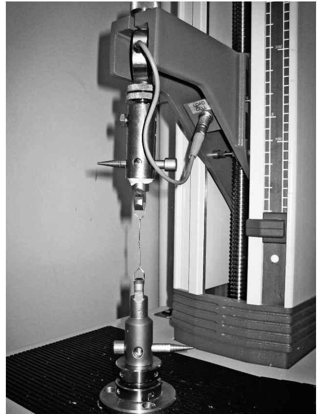
Figure 1. Customized jig used to test failure load.
